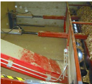
Figure 37. A hydraulic push bar unloader with auger conveyor. The fuel is pushed from the storage on the right side to the auger (EUBIONET2)
