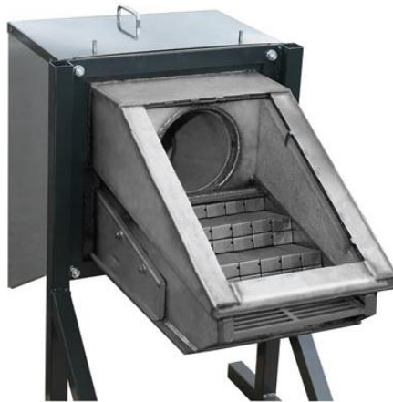
Figure 44. A moving grate system manufactured for the scale of 40–1,500 kW. A moving grate bio burner is designed to utilise several different kinds of solid bio fuels. The burner is able to use wood chip of varying quality, wood and peat pellets, peat and various agro biomasses. The grate of the burner is fully mobile and this enables the fuel to mix efficiently on its surface. The grate's mobility improves transport of the ash from the burning head to the ash compartment (Ariterm Group)
