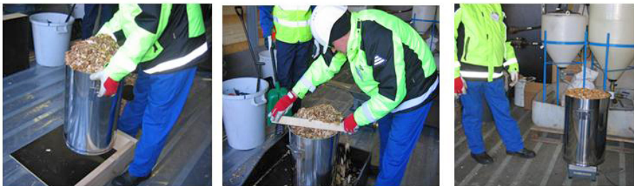
Figure 46. Fill the container (0.05 m 3 , 50 litres) and drop it freely from 15 cm height onto a wooden board. Repeat shock two times (photo on the left) and then remove surplus material by using a small scantling, which is shuffled over the container's edge in oscillating movements (photo in the middle). Weigh the container (photo on the right). The weight of the sample is the total weight minus the weight of the empty container (scaled earlier) (SolidStandards)
