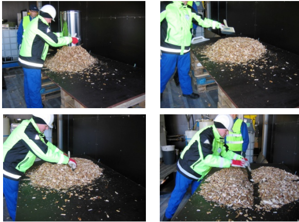
Figure 47. Corning and quartering for moisture content analysis. Divide as many times as needed to provide a sample for moisture content analysis (at least 300 g) (SolidStandards)
